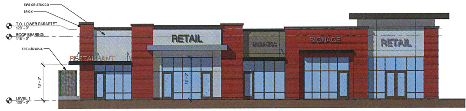
B2 NORTH EXTERIOR ELEVATION - BUILDING 1 1/8" = 1'-0"
