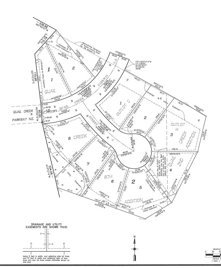
For the purposes of this plat, the North line of Outlot A, QUAIL CREEK 9TH ADDITION, is assumed to have a bearing of North 89 degrees 45 minutes 04 seconds East.
