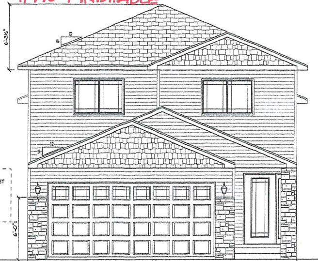
1 FRONT ELEVATION "C" SCALE: 1/4" = 1'-0" FINISHED SQ. FT. - (NOTE: SQ. FT. IS MEASURED FROM EXT. OF SHEATHING) 03:17 PM Wednesday, June 03, 2015
