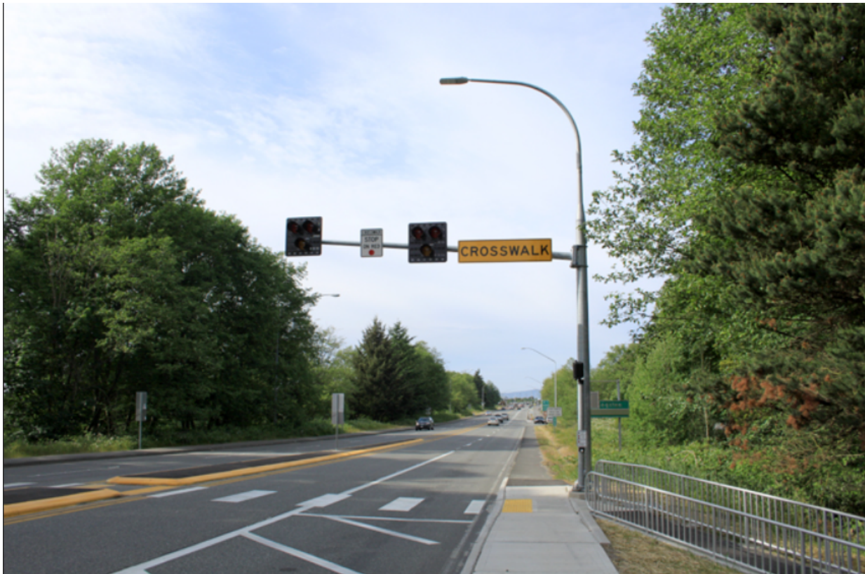
Figure 6: Pedestrian Hybrid Beacon (HAWK)
